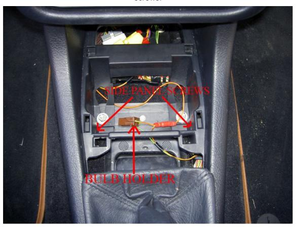
Now you can remove the two side panels. They just unclip, and need to be wiggled free. Once the panels have been removed, you need to remove the airduct pipes – again, they just unclip and pull off.
